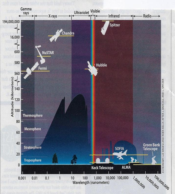
**RADIATION COLLECTORS.** Earth's atmosphere blocks most of the electromagnetic spectrum from reaching our planet's surface. This diagram shows the altitude in which the atmosphere absorbs half of the radiation at each wavelength in addition to where various telescopes observe that light. All observatories shown are currently operational.
